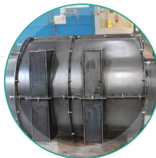
ContraTherm® pre-moulded insulation is engineered to match the dimensions of the component to be insulated.
